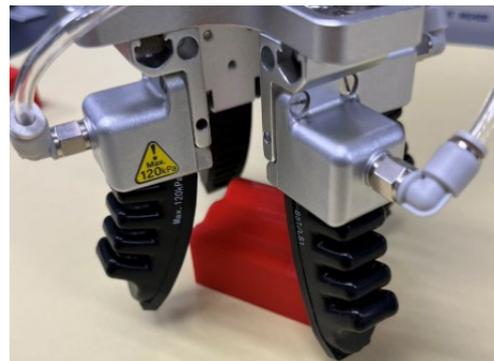
Fig. 1 MG400 with a soft gripper to pick various types of shapes.
