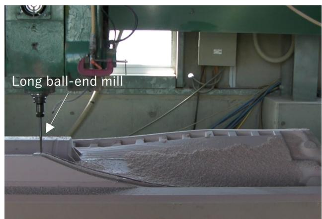
Fig.1 3D Machining scene of a large workpiece.
