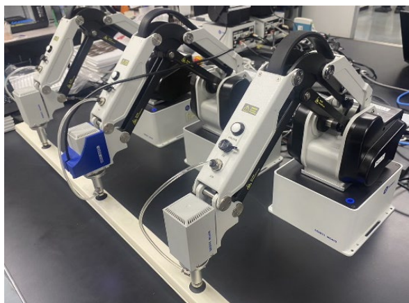
Fig. 1 Cooperative pick and place task using multiple robot MG400s .
