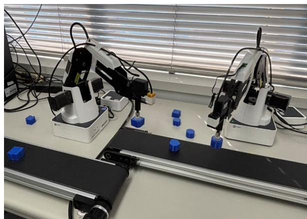
Fig. 2 Cooperative pick and place task using multiple robot Magicians , while checking defects.
