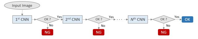
Fig. 1 Proposed cascade-type CNNs for binary classification of defective and non-defective.
